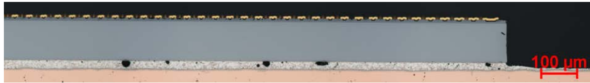
Figure 5: Cross section of SAC solder interface.
