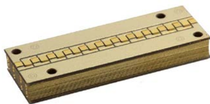
Figure 19: Single row emitter with 23 chips on the improved cooler delivering 200W cw laser output.
