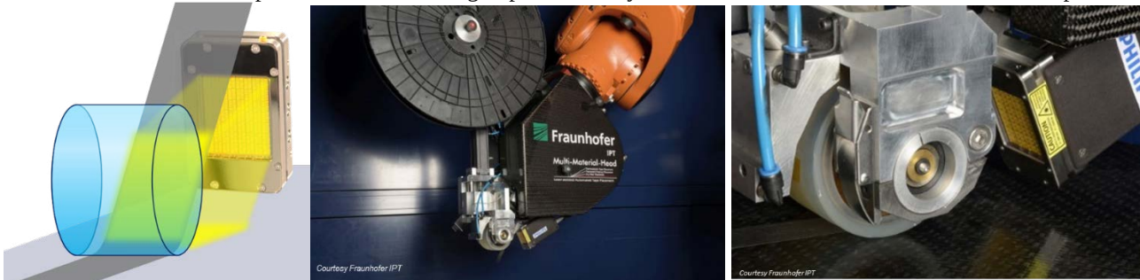
Figure 15: Welding of fiber-reinforced thermoplastic tapes with a VCSEL heating module. Left: Schematic. Middle: Integration on the automated tape-laying robot. Right: Close up of module and press wheel.
