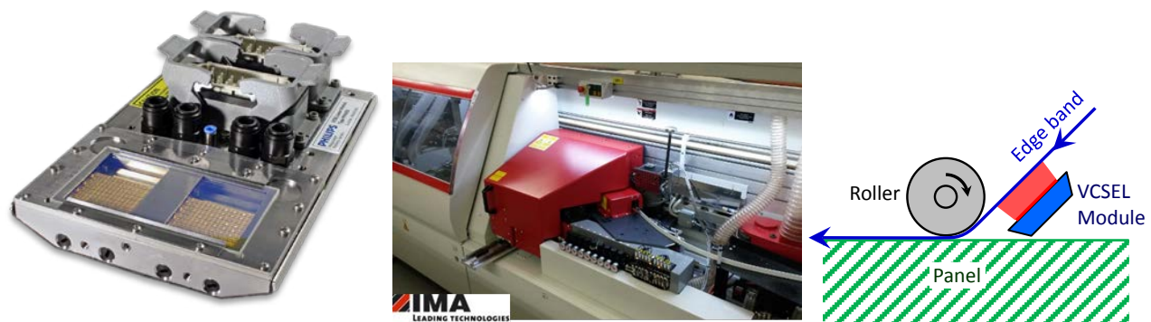
Figure 16: High power VCSEL product in a woodworking machine. Left: High power VCSEL system. Middle: Integration of the flat module into the equipment below the red hood. Right: Illustration of the process.
